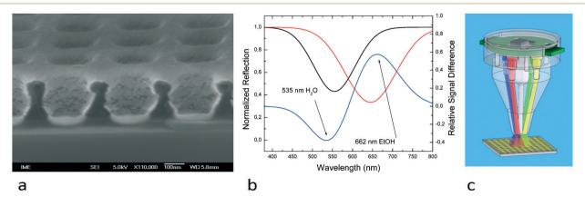
Fig. 5 (a) A scanning electron microscopy image of the substrate for measuring surface plasmon resonance. (b) Left axis: normalized amplitude of reflected light from the LSPR chip covered with H<sub>2</sub>O (black) or ethanol (red). Right axis: the blue line shows the difference between both curves. (c) CAD design of the LSPR head.
