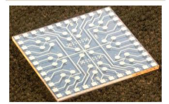
Fig. 7 A photograph of a 36-cell electrochemical chip
