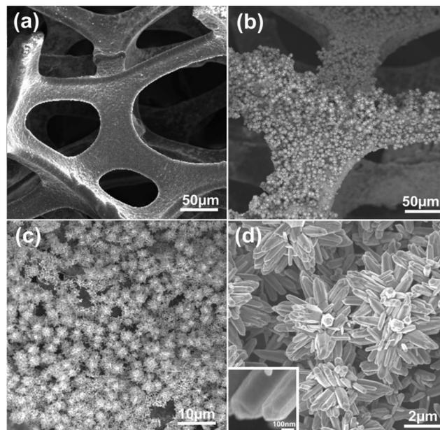
**Fig. 2** SEM images of the samples. (a) SEM image of 3D graphene foam. (b–d) SEM images of graphene/ZnO hybrids with different magnifications. The inset of (d) shows the morphology of a single ZnO nanorod at a high magnification.
