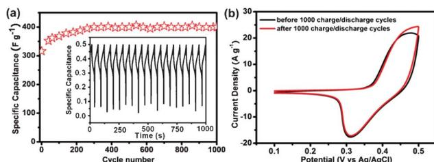
**Fig. 6** (a) The cycle performance of graphene/ZnO hybrid electrode at the current density of  $6.70 \text{ A g}^{-1}$  in  $2.0 \text{ M KOH}$  solution. The inset shows the charge–discharge profile for the graphene/ZnO hybrid electrode. (b) CV of graphene/ZnO hybrid electrode before and after 1000 charge–discharge cycles.
