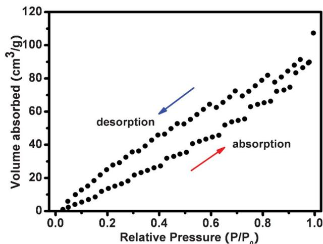
**Fig. 3** N<sub>2</sub> adsorption–desorption isotherm of a 3D graphene/ZnO hybrid.
