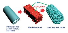
Fig. 4 Schematic view of morphology evolution of pristine stacked porous nanodisks.
