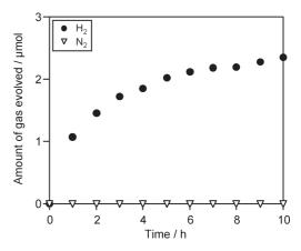
Fig. 1 Time course of photocatalytic evolution of H<sub>2</sub> using Pt (0.3 wt%)– TaON photocatalyst (0.2 g) suspended in a 5 mM NaI aqueous solution (pH 7 without adjustment) under visible light ( $\lambda > 420$  nm).
