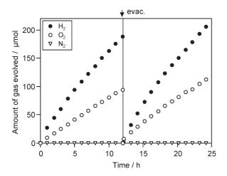
**Fig. 2** Time course of photocatalytic evolution of  $H_2$  and  $O_2$  using a mixture of Pt (0.3 wt%)–TaON (0.2 g) and Pt (0.5 wt%)–WO<sub>3</sub> (0.2 g) suspended in a 5 mM NaI aqueous solution (pH 7 without adjustment) under visible light ( $\lambda > 420$  nm).
