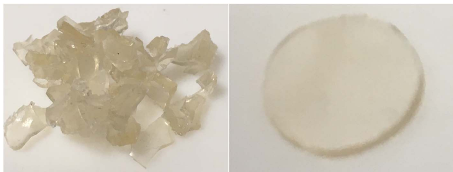
Fig. 11 Pictures of the cut pristine (left) and recast (at 120 °C) (right) dihydroxylated methyl erucate-based cross-linked HBPEs with 8 eq. of phenyl diboronic acid used as the cross-linker.
