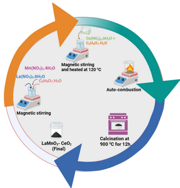
Fig. 1 A schematic of the autocombustion synthesis process of \text{LaMnO}_3\text{-CeO}_2 composites. Created with https://BioRender.com .
