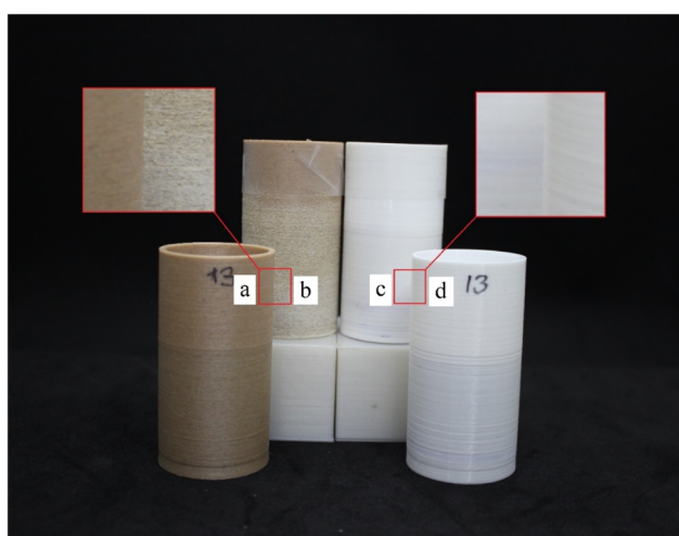
Fig. 4 Surface-activated and raw filters; (a) raw PLA/wood composite, (b) surface-activated PLA/wood composite, (c) surface-activated PLA, (d) raw PLA.
