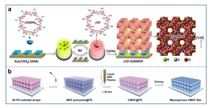
Fig. 3 (a) Preparation of \( \gamma CD-SURMOF \) membrane by assembly of metal ions and ligands layer by layer onto \( \gamma CD(SH)\_8 \) modified Au substrates. Reproduced with permission from ref. 29. Copyright 2022, Chinese Chemical Society. (b) Preparation of M-CMOF membranes with hierarchical porous structures by using PS arrays as templates. Reproduced with permission from ref. 30. Copyright 2024, American Chemical Society.
