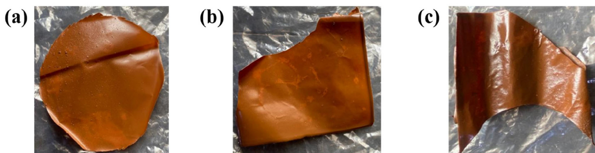
Fig. 7 Synthesized (a) MPVA/1BXT, (b) MPVA/3BXT and (c) MPVA/6BXT membranes.
