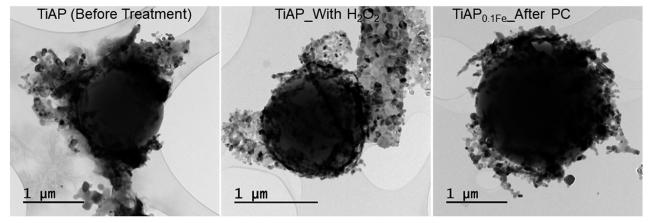
Fig. 4 Representative HR-TEM images of TiAP before treatment and samples with higher changes in the CI value (TiAP\_With H<sub>2</sub>O<sub>2</sub> and TiAP<sub>0.1Fe</sub>\_After PC).
