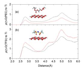
Fig. 4 RDFs simulated for  $TiO_2$ -filled PEC/LiTFSI SCE models between Ti atoms and oxygen atoms from (a) carbonyl groups in polymer chains and (b) TFSI anions. RDF curves are coloured based on salt concentration: 40 mol% (black) and 120 mol% (red).
