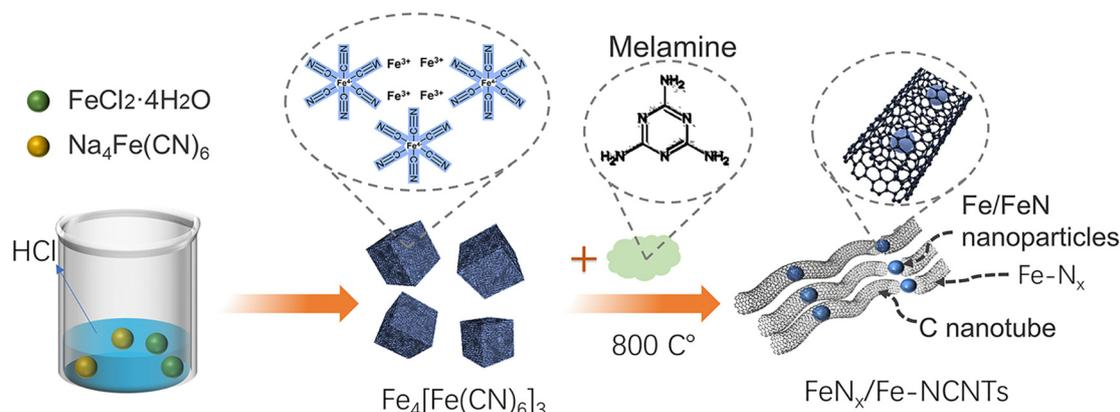
Fig. 1 Schematic diagram of the synthesis of FeN<sub>x</sub>/Fe-NCNTs.
