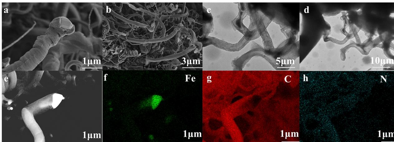
Fig. 4 (a) and (b) FESEM images of FeN<sub>x</sub>/Fe-NCNTs; (c) and (d) TEM images of FeN<sub>x</sub>/Fe-NCNTs; (e) EDS surface scan composition distribution of FeN<sub>x</sub>/Fe-NCNTs; (f) Fe; (g) C; (h) N.
