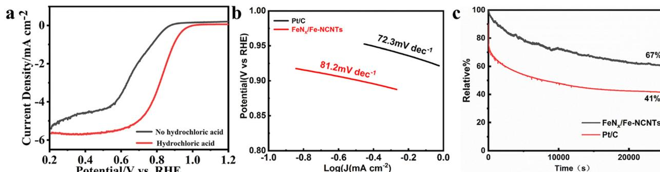
Fig. 6 (a) LSV curves of FeN<sub>x</sub>/Fe-NCNTs in the presence or absence of hydrochloric acid (1600 rpm); (b) Tafel slopes of FeN<sub>x</sub>/Fe-NCNTs and Pt/C catalysts; (c) chronoamperometry of FeN<sub>x</sub>/Fe-NCNTs and Pt/C at 0.6 V (vs. RHE).
