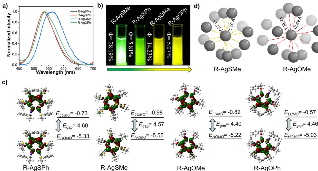
Fig. 3 (a) Photoluminescence (PL) spectra of *R*-type chiral silver nanoclusters *R*-AgSMe, *R*-AgSPh, *R*-AgOMe, and *R*-AgOPh. (b) Photoimages of *R*-AgSMe, *R*-AgSPh, *R*-AgOMe, and *R*-AgOPh clusters under 365 nm light. (c) DFT calculations of the LUMO/HOMO energy gap among the four *R*-type clusters *R*-AgSMe, *R*-AgSPh, *R*-AgOMe, and *R*-AgOPh. (d) Schematic diagram of *R*-AgSMe and *R*-AgOMe cluster stacking in the single crystal.
