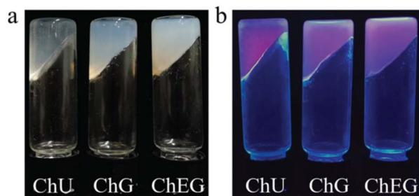
Fig. 26  $\text{Eu}^{3+}$  containing NaC–DES eutectogels without (left) and with (right) irradiation at  $\lambda = 365$  nm. Reproduced from M. Sun, Q. Li and X. Chen, Self-assembled luminescent cholate gels induced by a europium ion in deep eutectic solvents, *Soft Matter*, 2021, 17, 2815–2822 with permission from the Royal Society of Chemistry.
