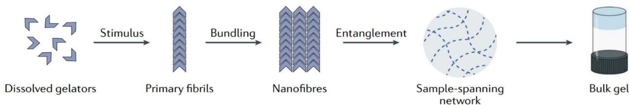
Fig. 5 Schematic of supramolecular gel assembly. Reproduced from P. R. A. Chivers and D. K. Smith, Shaping and structuring supramolecular gels, *Nat. Rev. Mater.*, 2019, 4, 463–478, <https://doi.org/10.1038/s41578-019-0111-6>. Copyright 2019, Springer Nature Limited.
