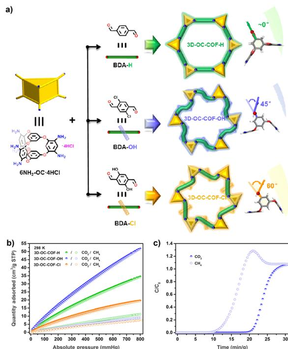
Fig. 11 (a) POC-based COFs containing different substituents; (b) N<sub>2</sub>, CO<sub>2</sub>, and CH<sub>4</sub> adsorptions of the three COFs at 298 K; (c) experimental column breakthrough curves for CO<sub>2</sub>/CH<sub>4</sub> (50 : 50, v/v) of 3D-OC-COF-OH at room temperature. Reproduced from ref. 90. Copyright 2021, The Chinese Chemical Society.
