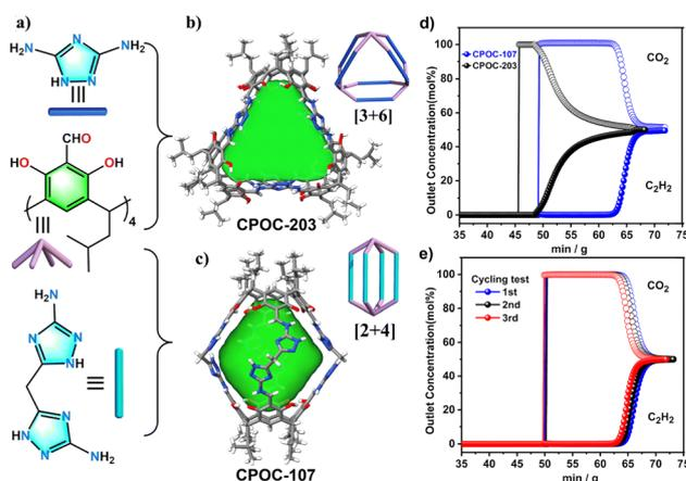
Fig. 9 (a–c) The chemical and crystal structures of CPOC-203 and CPOC-107; (d) experimental breakthrough curves for an equimolar mixture of C<sub>2</sub>H<sub>2</sub>/CO<sub>2</sub> at 298 K; (e) the recyclability of CPOC-107 under multiple mixed gas column breakthrough tests. Reproduced from ref. 84. Copyright 2023, The Royal Society of Chemistry.
