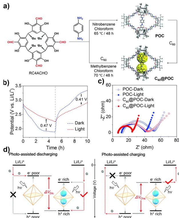
Fig. 16 (a) Schematic representation of the synthesis of POC and C<sub>60</sub>@POC; (b) charge and discharge curves of C<sub>60</sub>@POC with or without illumination; (c) Nyquist plots of POC and C<sub>60</sub>@POC with or without illumination; (d) schematic diagram of the photo-assisted Li-organic battery with POC and C<sub>60</sub>@POC cathodes. Reproduced from ref. 122. Copyright 2022, The Royal Society of Chemistry.
