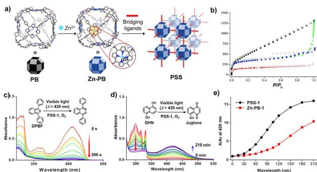
Fig. 4 (a) Construction of cage-based MOFs by using a porphyrin box; (b)  $\text{N}_2$  sorption isotherm at 77 K for 'PB' (red), 'PSS1' (black), 'PSS3' (green) and 'PSS4' (blue); electronic absorption spectra of DPBF (c) and DHN (d) in the presence of PSS-1,  $\text{O}_2$  and visible-light irradiation; (e) comparative catalytic performance of PSS-1 (black) and Zn-PB (red) for oxidation of DHN. Reproduced from ref. 57. Copyright 2018, The American Chemical Society.
