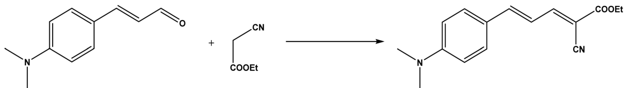
Fig. 28 Knoevenagel condensation of ( E )-3-(4-(dimethylamino)phenyl)acrolein and ethyl 2-cyanoacetate.
