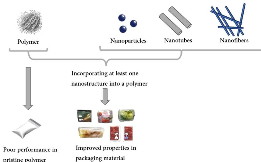
Fig. 1 Schematic representation of the overall procedure for the manufacturing of composites containing nanomaterials and enhancement of the functional properties.
