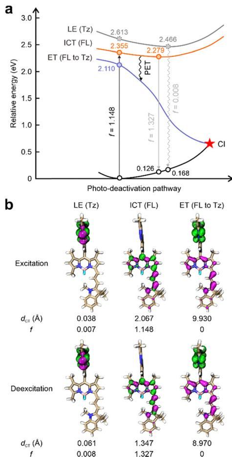
**Fig. 2** (a) Photoexcitation and deexcitation processes of **1** in dimethyl sulfoxide (DMSO). (b) Hole–electron distributions of different states with corresponding charge transfer distances ( $d_{CT}$ ) and oscillator strength ( $f$ ) values of **1** in DMSO. FL: fluorophore; Tz: tetrazine; LE: locally excited; ICT: intramolecular charge transfer; ET: electron transfer; PET: photoinduced electron transfer; electron: highlighted in green; hole: highlighted in pink.
