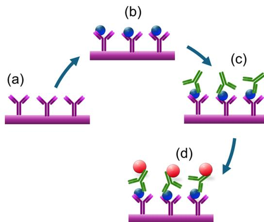
**Fig. 15** The schematic representation of the magneto-nanosensor biochip immunoassay involves several steps. (a and b) Immobilization of antibodies on the surface of the working electrode. (c) Sandwich structures are formed through the addition of biotinylated detection antibodies. (d) Magnetic nanoparticles bound to the detection antibodies generate a stray magnetic field that results in a change in sensor resistance due to the GMR effect.<sup>72</sup>
