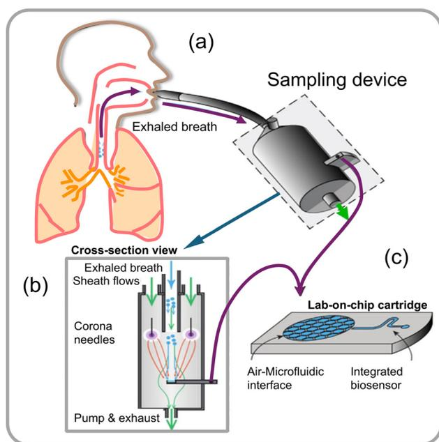
**Fig. 17** (a) Schematic illustration of a point-of-care (PoC) system designed for sampling aerosol from a high volume of air directly into a microfluidic device that captures exhaled breath condensate, (b) sampling device cross-sectional view integrated with a microfluidic detector, and (c) a lab-on-chip cartridge with a microfluidic interface that allows diagnosis from an exhaled-breath aerosol.<sup>86</sup>
