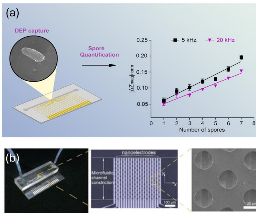
**Fig. 21** (a and b) A microfluidic device comprising 190 microwells and 20 aluminium nanoelectrodes adapted for performing dielectrophoresis (DEP) to capture spores, and the results of individual electrochemical impedance spectroscopy (EIS) measurements are shown in the line plot on right, enabling precise quantification. Reprinted with permission from ref. 89 (copyright open access © 2021 Published by American Chemical Society).
