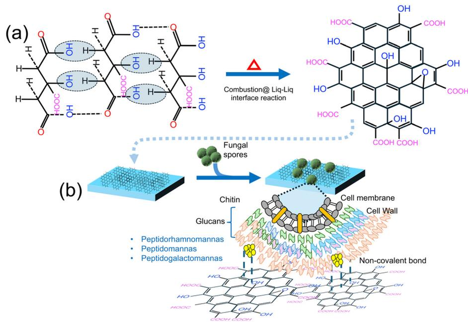
**Fig. 8** (a) Synthesis of the CD-based sensor film using flame/combustion at the liquid–liquid interface. (b) Schematic representation of fungal spore detection using the CD-based sensor film. Reprinted with permission from ref. 60 (copyright © 2019 Published by American Chemical Society).
