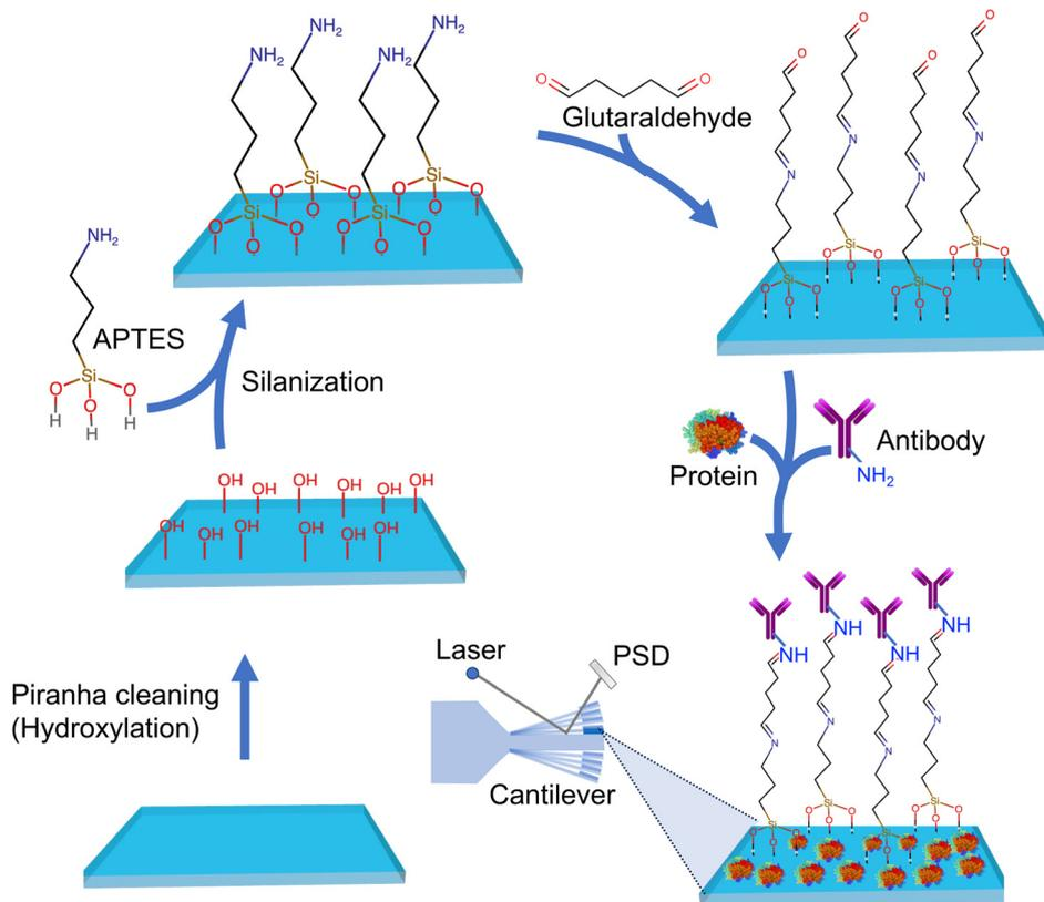
**Fig. 16** Scheme showing silicon microfabricated cantilever functionalization by treating the surface with APTES, glutaraldehyde followed by covalent attachment of anti-*Aspergillus niger* polyclonal antibodies ~IgG designed to capture fungal spores.<sup>73</sup> Binding of spores to the functionalized cantilever induces its deflection of the laser beam falling on it which is sensitively detected by the position sensitive detector (PSD).
