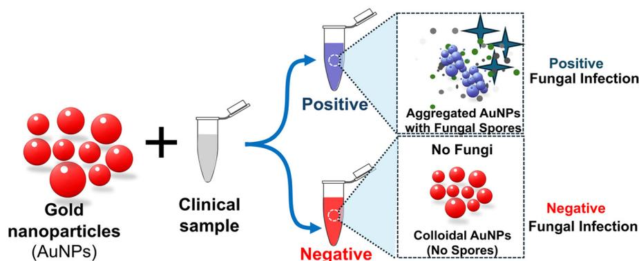
**Fig. 7** Schematic illustration of the gold nanoparticle system for plasmonic detection of fungi to facilitate self-diagnosis and hygiene control of clinical fungal infections. The progression in hue from red to pink to purple to blue signifies an escalation in the concentration of fungi present in a given clinical sample.<sup>59</sup>
