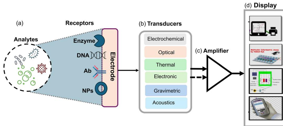
**Fig. 1** Schematic diagram illustrating the operational principle of a biosensor. This includes; (a) bio-recognition elements responsible for detecting specific analytes, such as viruses, bacteria or fungi; (b and c) signal generation components like transducers and an amplifier, which converts the recognized signals into a measurable data and; (d) display units that can be used to visualize the results generated by the biosensor.
