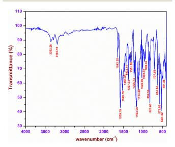
Fig. 3 FTIR spectrum of DMMA
