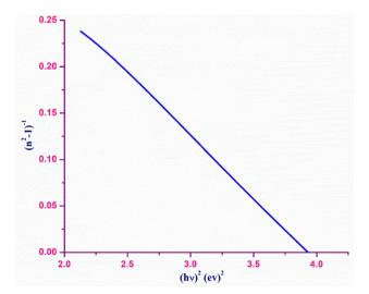
Fig. 7 Refractive index dispersion plot of the DMMA crystal using the Wemple-DiDomenico model.
