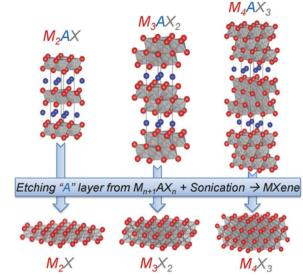
Fig. 2 Structures of MAX and the corresponding structures of MXenes. Reproduced with permission from ref. 61. Copyright 2014 Wiley.
