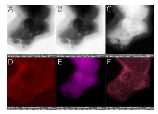
Fig. 2 STEM images of NG3 (5% GO) sample (A) brightfield, (B) darkfield, (C) high-angle annular dark-field imaging, and related element map (D) carbon (E) nickel (F) oxygen. Magnification: 760 000×, scale bar: 20 nm.
