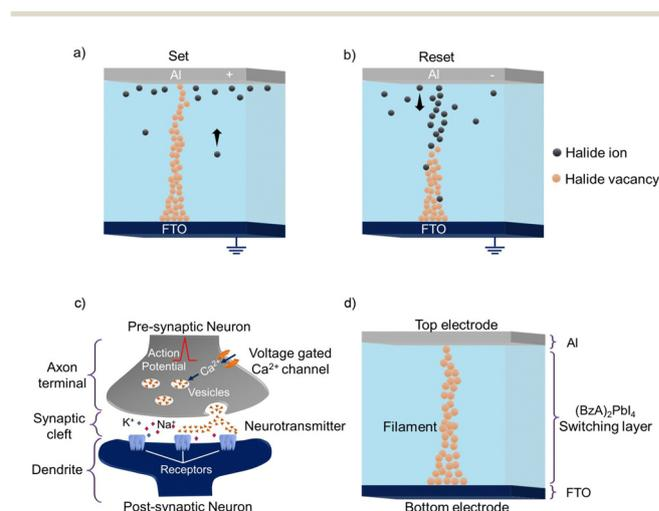
**Fig. 4** Resistive switching mechanism in layered hybrid perovskites. Schematic of (a) set (LRS) and (b) reset (HRS) switching governed by ion migration. Illustration of a (c) biological synapse and (d)  $(\text{BzA})_2\text{PbI}_4$ -based artificial synapse mimicking the biological function.
