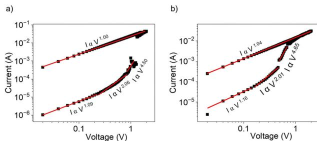
**Fig. 5** Conduction regimes in layered hybrid perovskite devices. (a) and (b) Linearly fitted current–voltage curves for LRS (top) and HRS (bottom) on a double logarithmic scale for a better understanding of the conduction mechanism related to the resistive switching in (a) bromide- and (b) iodide-based perovskite devices. The changes in slopes correspond to different conduction regimes.
