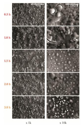
Fig. 8 Series of representative SEM images as a function of annealing at 500  $^{\circ}$ C with time from 0.5–3.0 hours shown at magnifications of 1k and 10k.
