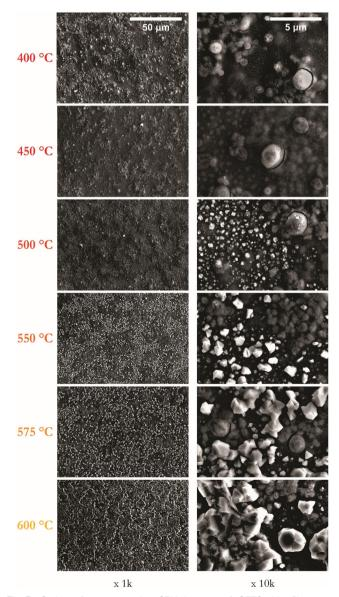
Fig. 3 Series of representative SEM images of CZTS thin films as a function of annealing temperature from 400 to 600 °C at 1 hour shown at magnifications of 1k and 10k
