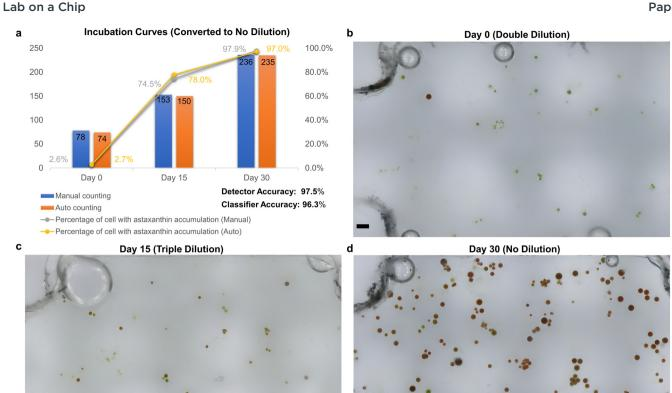
Fig. 5 Monitoring the accumulation of astaxanthin in Haematococcus Pluvialis. a) Culture experiment data and comparison graph of manual and AIMP obtained statistics. Example images of a single observation chamber at b) day 0 (samples are diluted twofold before adding to the chip), c) day 15 (samples are tripled diluted before adding to the chip), and d) day 30 (samples are not diluted). Scale bars are 200 µm.
