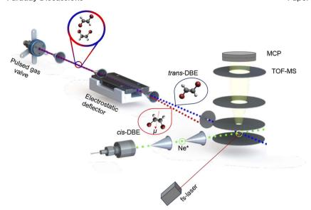
Fig. 1 Schematic of the crossed-molecular-beam experiment used in the present study. The polar *cis* and apolar *trans* stereoisomers of 1,2-dibromoethene (DBE) were separated from a mixture using an electrostatic deflector and overlapped with a second beam containing metastable neon atoms (Ne\*) in the extraction region of a time-of-flight mass spectrometer (TOF-MS) to study isomer- and rotationally-resolved chemi-ionisation (CI) reactions. See text for details.
