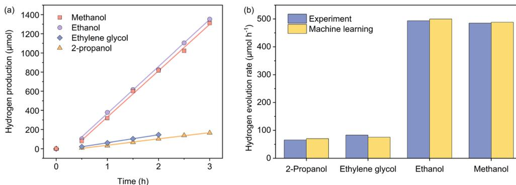
**Fig. 5** (a) Kinetics of photocatalytic hydrogen evolution carried out independently under four experimental conditions as suggested by the machine learning model, involving 2-propanol (Cond. 1), ethylene glycol (Cond. 2), ethanol (Cond. 3), and methanol (Cond. 4). Please refer to Table 3 for specific experimental parameters associated with each condition. (b) Comparisons between the actual and predicted hydrogen evolution rates under the four named conditions.
