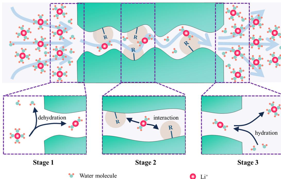
**Fig. 1** The three stages of ion passing through the membrane. Stage 1 is the entering process of ions into the membrane, during which partial dehydration occurs. Stage 2 is the ion diffusion inside the membrane, during which ions may interact with functional groups on the membrane. Stage 3 is the returning of ions from the membrane to the solution on the other side, during which hydration of ions may occur.
