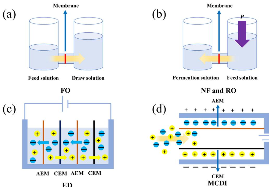
**Fig. 2** Schematic diagram of different driving forces corresponding to technology. (a) FO technology (osmotic pressure driving); (b) NF technology and RO technology (hydraulic driving); (c) ED technology (electric potential driving); (d) MCDI technology (electric potential driving).
