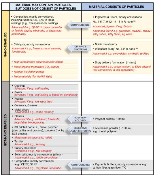
Fig. 2 Categories with examples sorted according to the three dimensions of the AMEA framework. Advanced materials or advanced processes are listed in italic red font; manufacturing processes are indicated as arrows. This categorization leads to four quadrants for each of which Fig. 3 provides assessment recommendations. See Glossary for abbreviations.
