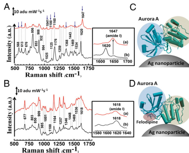
Fig. 33 SERS study of specific binding of felodipine to Aurora A. (A) SERS spectrum of Aurora A (black) and Aurora A complexed with felodipine (red). (B) SERS spectrum of Aurora B (black) and after treatment with felodipine (red). From ref. 228.
