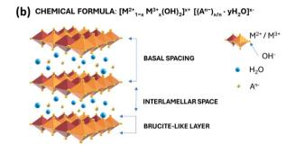
Scheme 2 Crystal structures of an (a) MXene and (b) LDH.
