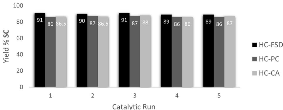
Fig. 9 Recycling catalytic test for the coupling of SO and CO<sub>2</sub> catalyzed by HC-FSD, HC-PC and HC-CA. Reaction conditions: 0.875 mmol SO (100 μL), autoclave, *p* (CO<sub>2</sub>) 3 bar, catalyst loading 10 wt%, temperature 70 °C, 7 h. Isolated yields are given, after purification of the reaction crude by flash column chromatography. Yield of SC was the average after two runs. Selectivity was > 99% for all catalytic runs.
