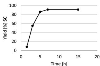
Fig. 8 Reaction rate for the conversion of SO into SC catalyzed by HC-FSD. Reaction conditions: 0.875 mmol SO (100  $\mu$ L), autoclave. Isolated yields after purification of the reaction crude by flash column chromatography. Yields are expressed as mean of two independent replicates. Selectivity was always >99%.
