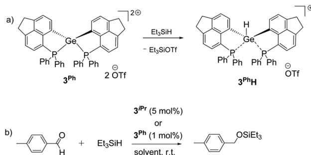
Scheme 3 (a) Si–H bond activation by  $3^{\text{Ph}}$  leading to  $3^{\text{Ph}}\text{H}$  within 24 hours; (b) hydrosilylation of *p*-methyl benzaldehyde using  $3^{\text{iPr}}$  or  $3^{\text{Ph}}$  as the catalyst (see the ESI† for the detailed spectroscopic and experimental procedures of each reaction).
