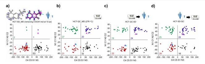
Fig. 5 2D plot of N-C-N-C and C-C-S-N dihedral angle distributions of: (a) polyamorph I obtained by SD; (b) polyamorph II obtained by QC; (c) SD of polyamorph II; and (d) QC of polyamorph I. HCT structures representative of each dihedral angle combinations is also presented. The blue triangle corresponds to the structure in  $P2_1$  space group while the pink triangle corresponds to the other polymorph in  $P2_1/c$  space group. EtOH stands for ethanol.
