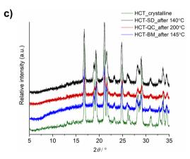
Fig. 2 (a) mDSC thermograms of HCT polyamorphs obtained by SD, QC and BM after a second heating cycle (total heat flow); (b) mDSC (total and reversing heat flow) and TGA of polyamorph I (obtained by SD) after the second heating cycle; (c) PXRD data of all HCT polyamorphs obtained after the recrystallization temperature.
