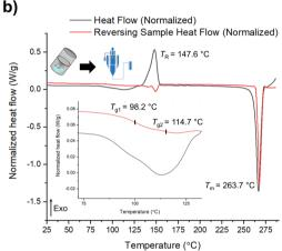
Fig. 3 mDSC data of (a) SD of polyamorph II obtained by QC; and (b) SD of polyamorph III obtained by BM.
