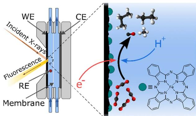
Fig. 1 Schematic side view of the electrochemical cell and simplified CO<sub>2</sub> reduction process on the surface of the working electrode. The dark green circles represent iron phthalocyanine (FePc), the molecular catalyst used in this study, whose structure is shown in the right corner. WE, CE, and RE stand for "working electrode", "counter electrode", and "reference electrode", respectively. The scheme is not drawn to scale.
