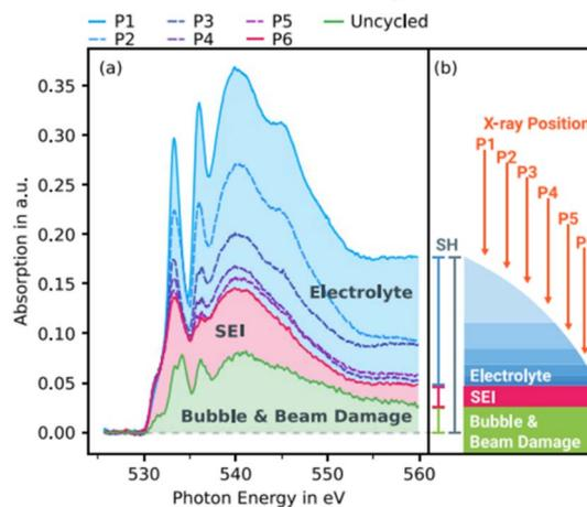
Fig. 5 (a) Illustration of a novel approach to investigate the SEI on silicon thin-film electrodes *in situ* through transmission sXAS and (b) extraction of the SEI spectrum from the overshadowing electrolyte spectrum and subtraction of the bubble and beam damage.<sup>82</sup>
