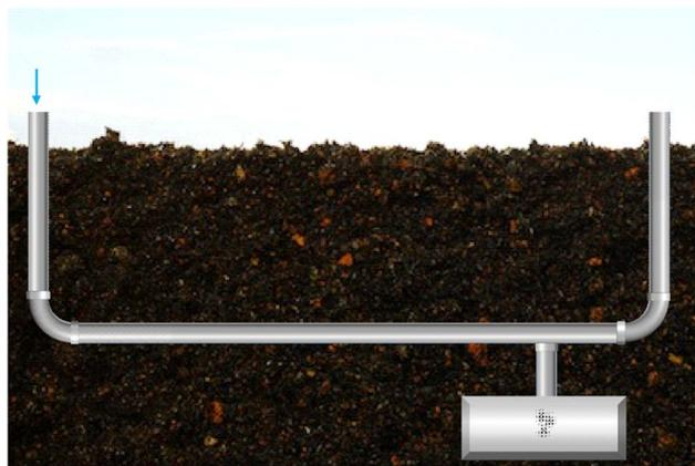
Fig. 13 Schematic of condensation drinking water production method.
