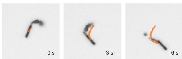
**B** Instantaneous velocities of MnO<sub>2</sub> micromotors at 2 wt. % H<sub>2</sub>O<sub>2</sub>
