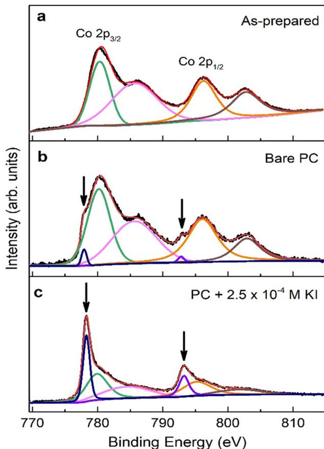
Fig. 5 X-ray photoelectron spectra of Co  $2p_{3/2}$  and Co  $2p_{1/2}$  for (a) as-prepared, (b) treated in bare PC and (c) PC +  $2.5 \times 10^{-4}$  M KI samples. The downward arrows point to the Co  $2p_{3/2}$  and Co  $2p_{1/2}$  peaks of metallic Co (in blue and purple in (b) and (c)). Additionally, green and orange correspond to  $\text{Co}^{2+}$ , and pink and brown to  $\text{Co}^{3+}$ . Solid black lines are experimental data, whereas solid red lines refer to fitting spectra.
