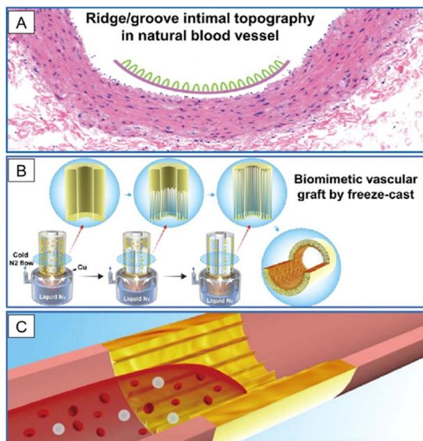
**Fig. 6** Application of nanolamellar films in SDVGs. (A) Natural blood vessel shows a ridge/groove nanotopography on the intimal surface. (B) SDVG with a biomimetic structure is prepared by applying a freeze-cast technique with lamellar nanotopography on the inner surface. (C) VG is used to replace the injured vessel to promote fast endothelialization and to maintain long-term patency. Reprinted with permission from ref. 70. Copyright 2019, American Chemical Society.
