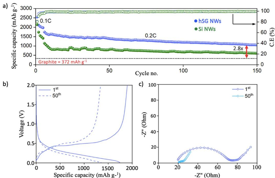
Fig. 3 (a) Cyclic performance of hSG NWs and Si NWs at 0.2C cycled between 0.011–2.0 V, (b) corresponding voltage–specific capacity plot and (c) EIS analysis of hSG NWs after 1<sup>st</sup> and 50<sup>th</sup> cycle of hSG NWs.
