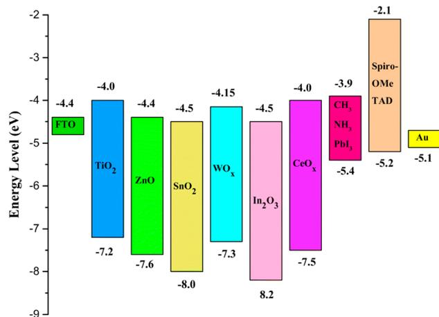
Fig. 19 Energy zones of diverse materials used as inorganic ETM in different films of PSCs (reproduced with permission from ref. 166. Copyright 2018 Springer).
