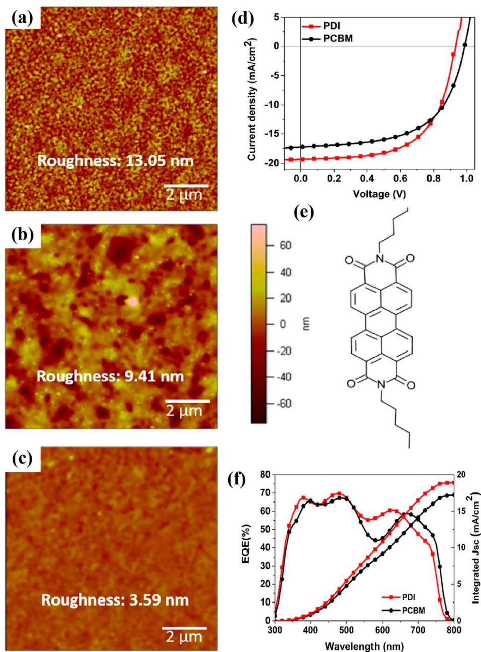
Fig. 18 AFM pictures of perovskite absorber ( $\text{CH}_3\text{NH}_3\text{PbI}_{3-x}\text{Br}_x$ ) (a) prepared on PEDOT:PSS film, (b) after fabrication of PCBM, and (c) PDI film on PEDOT:PSS/perovskite thin layer. (d)  $J$ - $V$  curves, (e) PDI molecular assembly, and (f) EQE-wavelength findings for both PCBM and PDI ETL-based PSCs (reproduced with permission from ref. 164. Copyright 2017 Elsevier).
