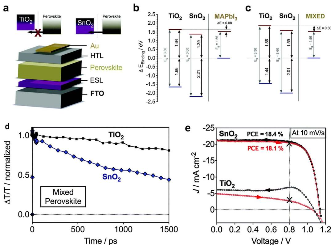
Fig. 21 (a–c). Diagram of energy level plans and electron inoculation properties of SnO<sub>2</sub>- and TiO<sub>2</sub>-based planar PSCs, (d) transient absorption findings, (e) current–voltage ( $J$ – $V$ ) curves of TiO<sub>2</sub>- and SnO<sub>2</sub>-based planar mixed halide-mixed cation PSCs (reproduced with permission from ref. 184. Copyright 2015 RSC).
