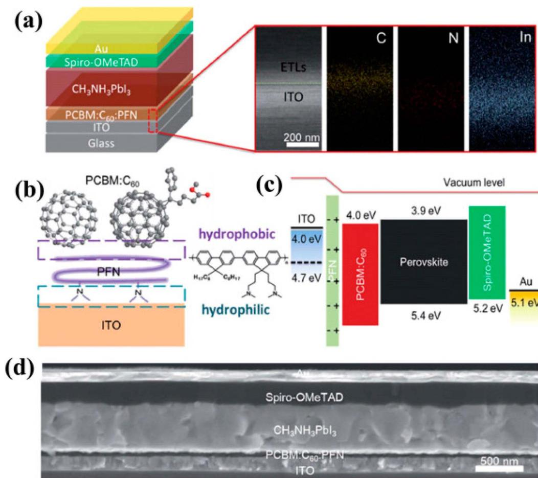
Fig. 16 (a) Illustrative depiction of the produced thin-film assembly and SEM image with EDS plotting of the cross-section of ITO/PCBM:C<sub>60</sub>:PFN (approx 120 nm). (b) Symbolic drawing of vertical phase parting in the ternary PCBM:C<sub>60</sub>:PFN and molecular structure of PFN. (c) Energy figure, and (d) SEM image showing the side view of the established device (reproduced with permission from ref. 159. Copyright 2018 RSC).
