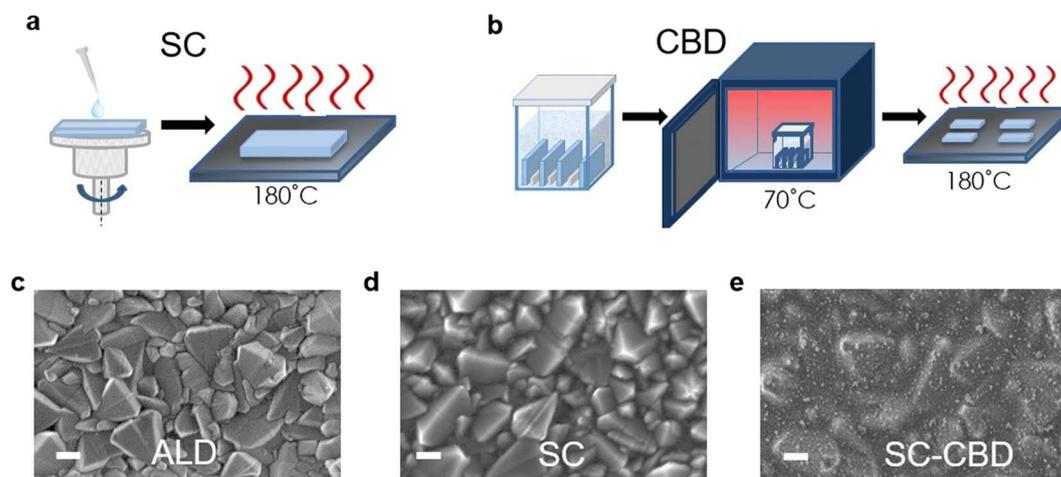
Fig. 22 Symbolic diagram showing the preparation of SnO<sub>2</sub> thin layers using (a) spin coating (SC) and (b) chemical bath deposition (CBD). (c) Top-view SEM pictures of SnO<sub>2</sub> films prepared by atomic layer deposition (ALD), (d) spin coating (SC), and (e) spin coating and chemical bath deposition (SC-CBD). All scale bars are 200 nm (reproduced with permission from ref. 74. Copyright 2016 RSC).
