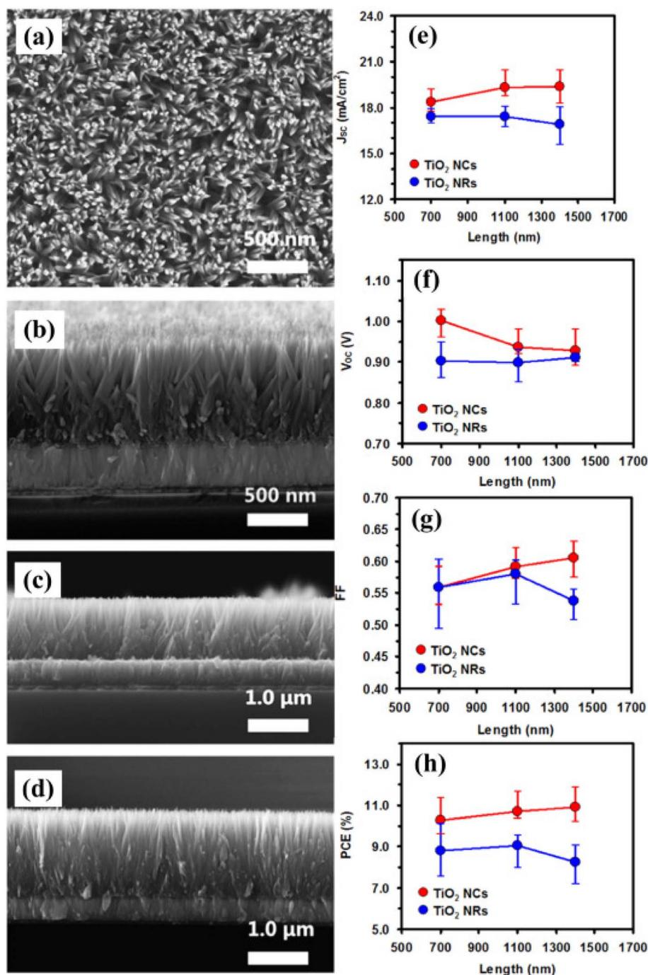
Fig. 12 (a) Top view of nanocones and (b) side view of SEM image of TiO<sub>2</sub> nanocones grown over FTO glass substrate (a and b) with 700 nm, (c) 1100 nm, (d) 1400 nm, TiO<sub>2</sub> nanocones. Comparative works of both TiO<sub>2</sub> nanocones and nanorods for 16 devices having various physical parameters (e) J<sub>sc</sub>, (f) V<sub>oc</sub>, (g) FF, and (h) PCE of PSCs with respect to length (reproduced with permission from ref. 139. Copyright 2015 Elsevier).
