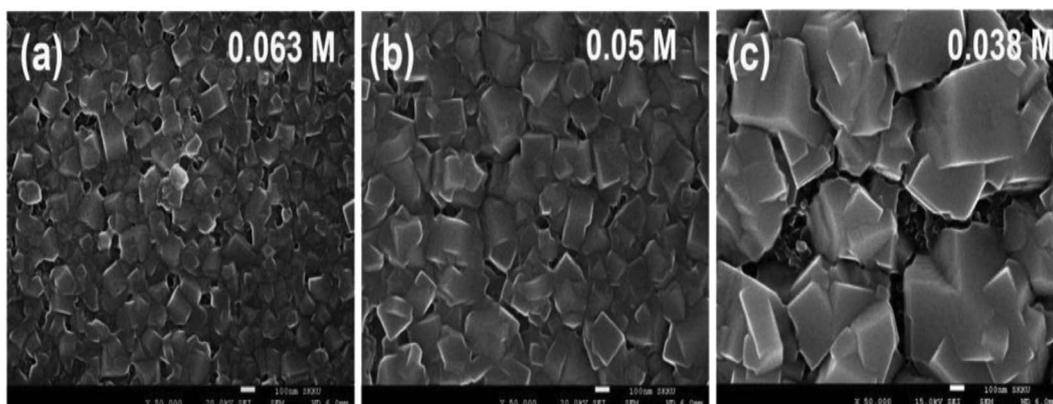
Fig. 24 SEM images for  $\text{CH}_3\text{NH}_3\text{PbI}_3$  produced via two-step spin-coating with (a) 0.063 M, (b) 0.05 M, and (c) 0.038 M  $\text{CH}_3\text{NH}_3\text{I}$  solution. Scale bars signify 100 nm (reproduced with permission from ref. 200. Copyright 2014 NPG).
