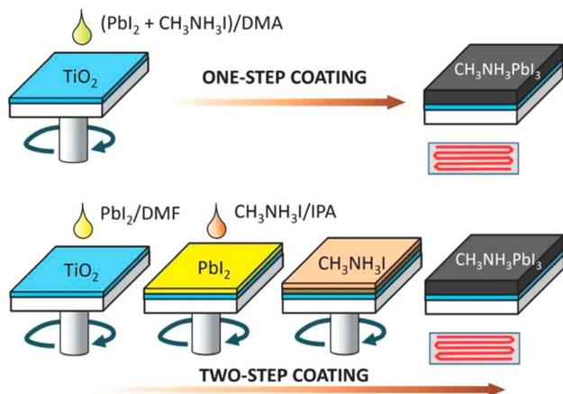
Fig. 23 One-stage and two-stage coating methods to prepare  $\text{CH}_3\text{NH}_3\text{PbI}_3$  perovskite layers. DMA, DMF, and IPA signify dimethyl acetamide, dimethyl formamide, and isopropyl alcohol, respectively (reproduced with permission from ref. 197. Copyright 2014 AIP).
