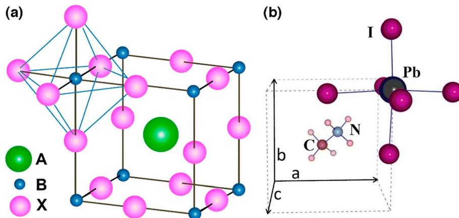
Fig. 1 (a)  $ABX_3$  perovskite construction presenting  $BX_6$  octahedral and bigger A cations engaged in the cuboctahedral place. (b) The element cell of cubic  $MAPbI_3$  perovskite (reproduced with permission from ref. 25, copyright 2015 Elsevier).
