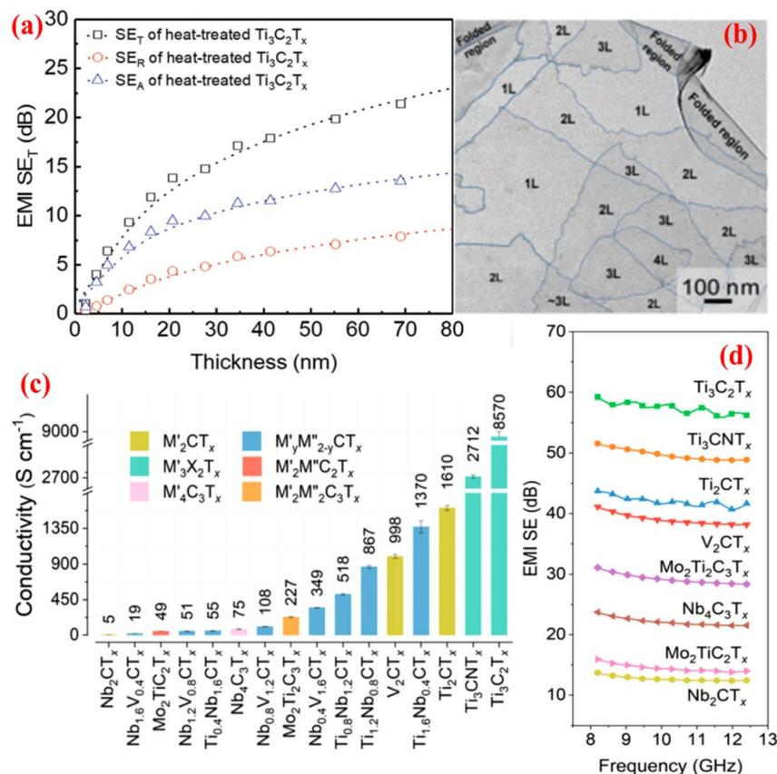
Fig. 2 (a) EMI SE values of  $\text{Ti}_3\text{C}_2\text{T}_x$  film after annealing at  $400\text{ }^\circ\text{C}$  and (b) transmission electron microscopy image of few-layer thick MXene film. Reproduced with permission from ref. 62 with permission from Wiley-VCH Verlag GmbH & Co. KGaA, Weinheim, © 2020. (c) Conductivity and (d) EMI SE of  $5\text{ }\mu\text{m}$ -thick MXene films with different compositions. Reproduced from ref. 63 with permission from the American Chemical Society, © 2020.
