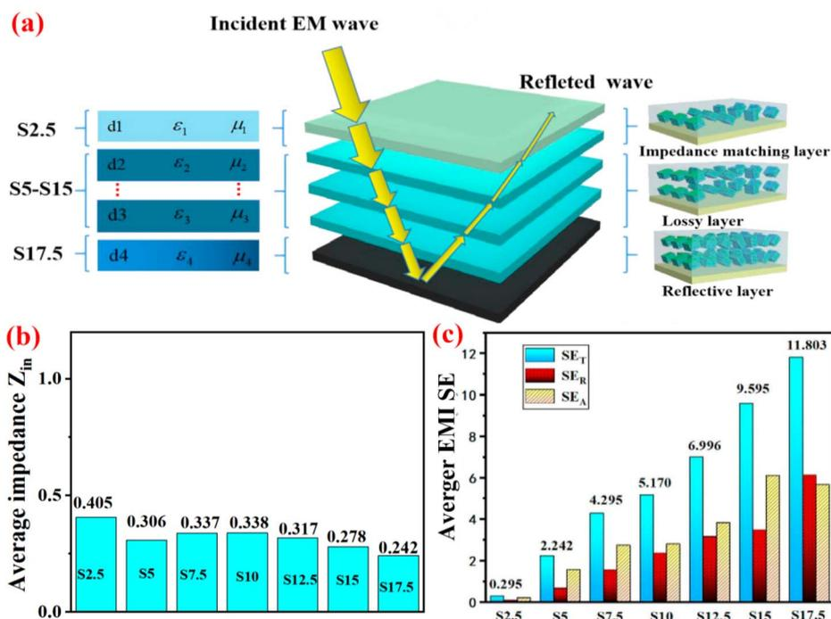
Fig. 12 (a) Multilayer impedance gradient structure consisting of  $Ti_3C_2T_x$  MXene/polymer films; (b) the average impedance  $Z_{in}$  of S2.5–S17.5; (c) the average sEMI SE of the samples S2.5–S17.5. Reproduced from ref. 186 with permission from Elsevier Ltd., © 2021.
