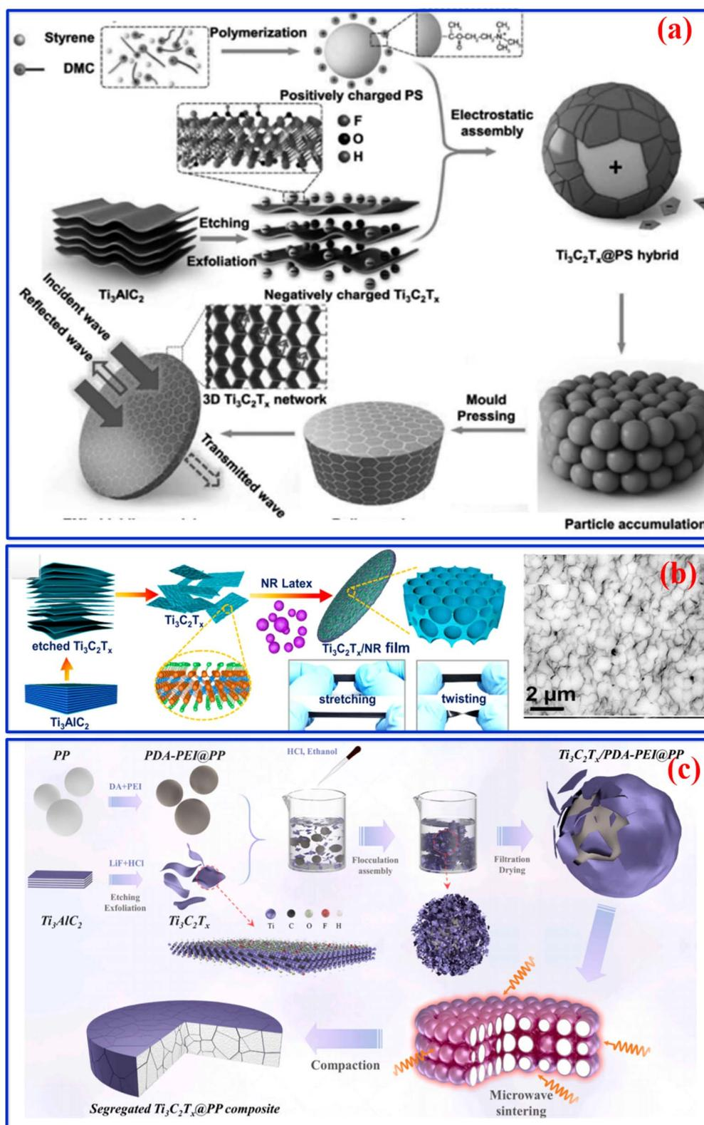
Fig. 7 Fabrication of MXene/polymer composites with segregated and hybrid structures. (a) Segregated  $Ti_3C_2T_x$ /polypropylene composite. Reproduced from ref. 123 with permission from Wiley-VCH Verlag GmbH & Co. KGaA, Weinheim, © 2017. (b) Segregated MXene@NR film. Reproduced from ref. 138 with permission from Elsevier Ltd., © 2019. (c) Segregated  $Ti_3C_2T_x$ @polystyrene nanocomposite. Reproduced from ref. 139 with permission from Elsevier B.V., © 2021.
