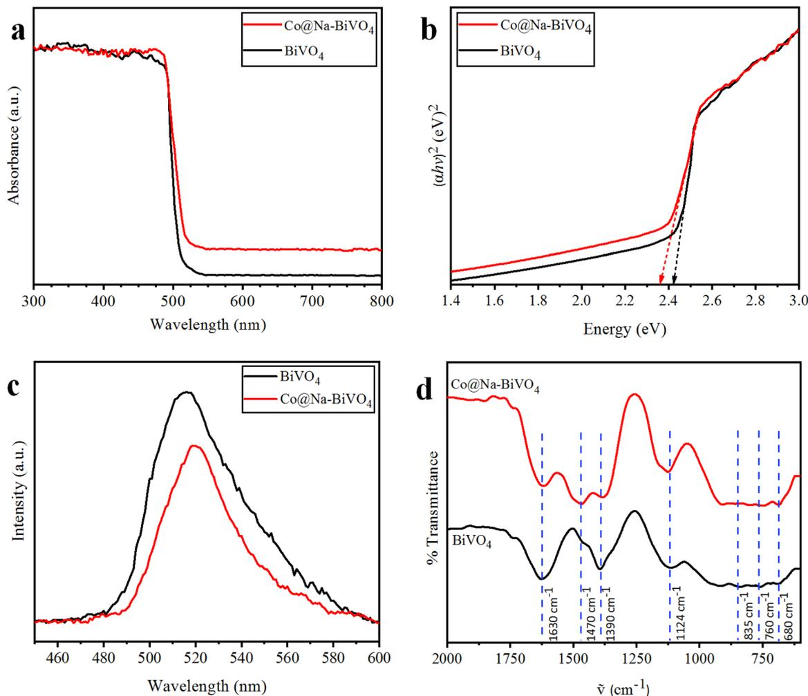
Fig. 5 (a) UV-vis/DRS, (b) energy diagram, (c) PL spectra (both catalysts at the same concentration in ethanol) and (d) FT-IR spectra of the as-synthesized  $\text{BiVO}_4$  and  $\text{Co@Na-BiVO}_4$  (powders compressed into KBr pellets).
