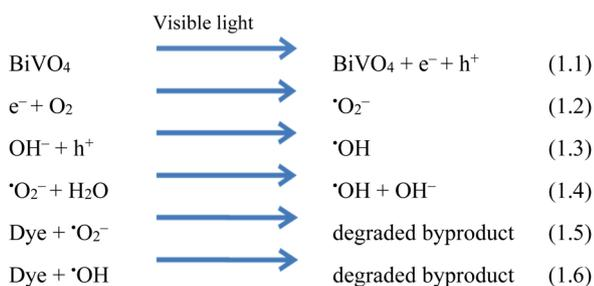
Scheme 1 Photocatalytic reactions involved in dye degradation.
