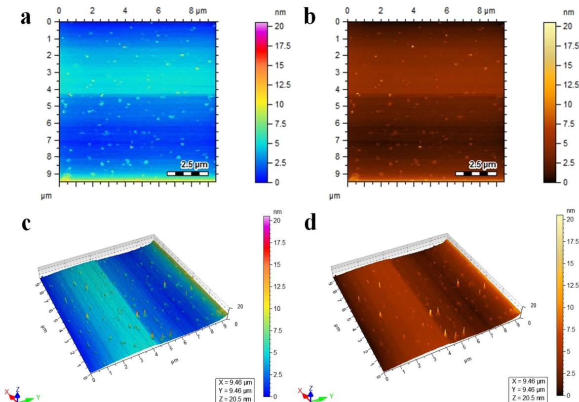
Fig. 4 AFM images of Co@Na-BiVO<sub>4</sub> (a and b) topographical images, and (c and d) three-dimensional view.
