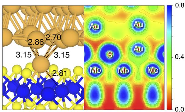
Fig. 3 Optimized geometry of the  $\text{Au}_5$  interface (left image), in the proximity of the contact area. Relevant Au–Mo and Au–Au bond lengths (in angstrom) are shown. Contour plot of the ELF for the  $\text{Au}_5$  interface (right image) in the proximity of the contact area. The color scheme is RGB, and red corresponds to  $\text{ELF} = 0$ , whereas blue to  $\text{ELF} = 0.8$ .
