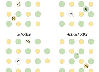
Fig. 1 (a) Perfect crystal of a square metal iodide lattice MI. (b) Electronic disorder involving electronic defects e' and h\*. (c) Different types of ionic disorder involving metal and iodide point defects (interstitials  $I_i'$  and  $M_i^{\bullet}$  and vacancies  $V_I^{\bullet}$  and  $V_M'$ ).
