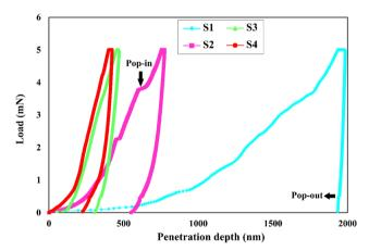
The load-displacement curves of the electrodeposited specimens.
