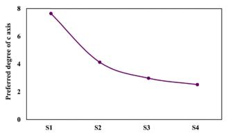
Fig. 3 The preference degrees of the electrodeposited coatings to grow along the c-axis.
