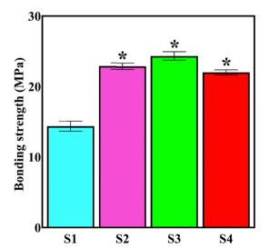
Coating-substrate adhesion strength values (\*p < 0.0001 vs. S1).
