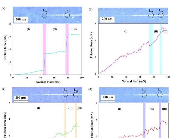
Fig. 10 Obtained curves from nanoscratch testing along with the corresponding panorama images of track traces (at the magnification of  $100 \times$ ): (a) S1, (b) S2, (c) S3, and (d) S4.
