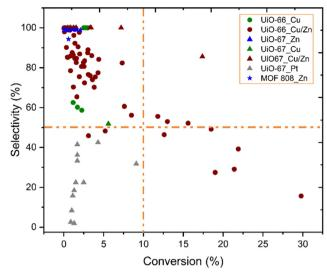
Fig. 10 Selectivity toward methanol versus conversion of CO2. While different symbols represent various metal-organic frameworks, different colours represent various incorporated metal active sites. 37-46 Orange dashed lines represent 10% conversion and 50% selectivity and have been included to guide the eyes.
