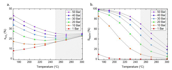
Fig. 2 Influence of pressure and temperature on (a) equilibrium conversion of  $CO_2$  and (b) selectivity toward methanol at equilibrium. The dashed area indicates the temperature range typically applied for  $CO_2$  hydrogenation to methanol in industry. The ratio of  $H_2/CO_2$  was 3:1, and methane was excluded from the calculations. Factsage was used for the analyses.<sup>55</sup>
