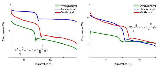
DSC curves (2nd heating scan) of the different PHUs obtained from functionalized vanillin bis-carbonates.
