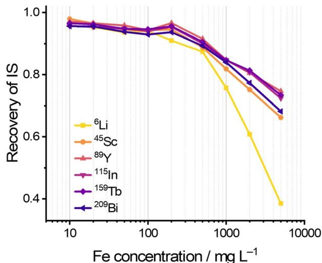
Fig. 4 Intensity recovery of <sup>45</sup>Sc, <sup>89</sup>Y, <sup>115</sup>In, <sup>159</sup>Tb, and <sup>209</sup>Bi in 2% HNO<sub>3</sub> with different Fe concentrations in relation to the IS solution with no matrix.
