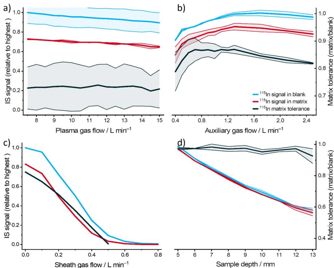
Fig. 2 Relative signal intensities of <sup>115</sup>In in blank and matrix solutions (relative to the highest signal in the blank), and the corresponding matrix tolerance obtained using different (a) plasma gas flows, (b) auxiliary gas flows, (c) sheath gas flows, and (d) sample depths. The lines with light color represent the standard deviation of the measurement.
