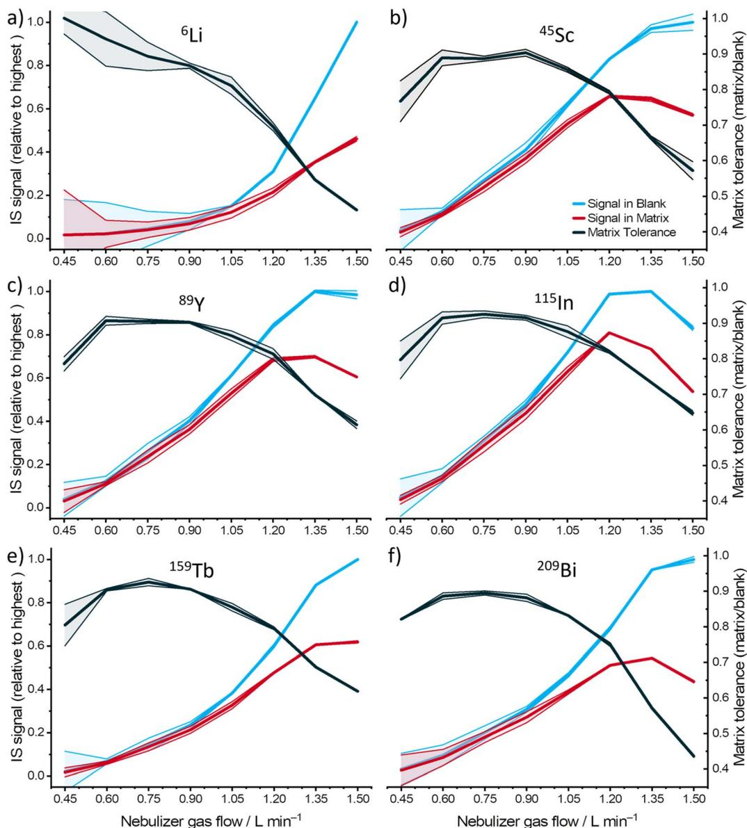
Fig. 1 Relative signal intensities of (a) <sup>6</sup>Li, (b) <sup>45</sup>Sc, (c) <sup>89</sup>Y, (d) <sup>115</sup>In, (e) <sup>159</sup>Tb and (f) <sup>209</sup>Bi in blank and matrix solutions (relative to the highest signal in the blank), and the corresponding matrix tolerance obtained using different nebulizer gas flow rates. The lines with light color represent the standard deviation of the measurement.
