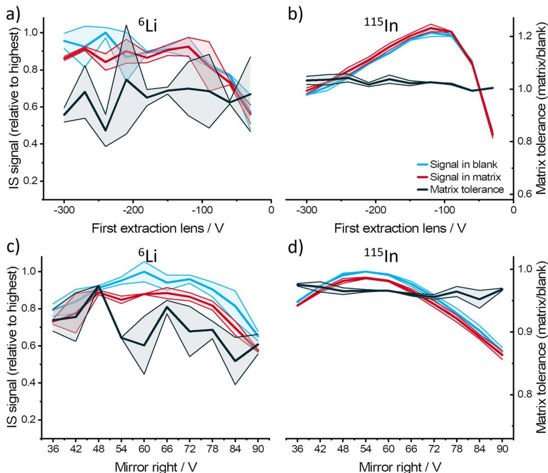
Fig. 3 Relative signal intensities of  $^6\text{Li}$  and  $^{115}\text{In}$  in blank and matrix solutions (relative to the highest signal in the blank), and the corresponding matrix tolerance obtained using different (a and b) first lens voltages and (c and d) right mirror voltages. The lines with light color represent the standard deviation of the measurement.
